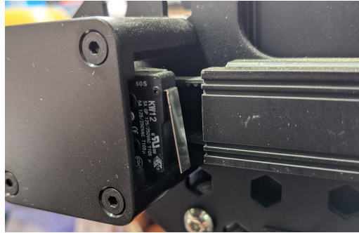
Figure 2.10: Mechanical Limit Switch on 3D Printer (x-axis)
